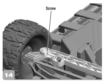
• Insert a screw through the large opening in the steering column cap and the hole in the steering column. Tighten the screw.
